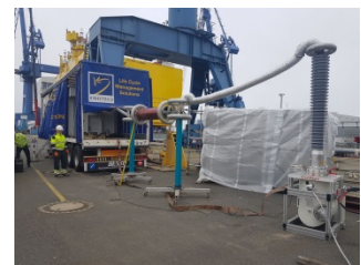
The HV installation was tested with a resonance testing system from an external testing institute.
